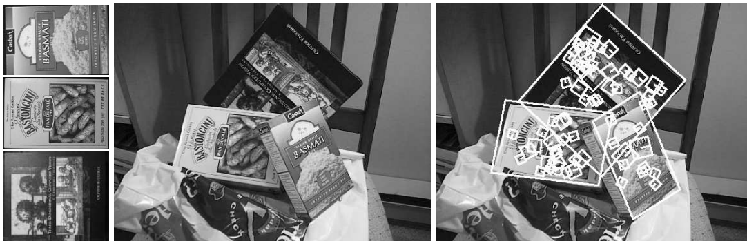
Figure 2.2: Model images of planar objects are shown in the left column of images. Recognition results to the right show model outlines and image keys used for matching. [Lowe 1999]
