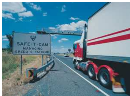
Figure 1.3: The Safe-T-Cam system uses computer vision to monitor heavy vehicle lane positioning and speed, improving the safety of road travel.
