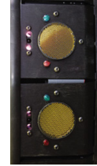
Ultrasound time-of-flight & Infrared reflected-intensity
